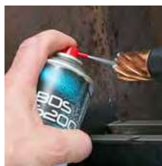
Step 1: Prior to drilling, spray high-performance lubrication spray directly into the drill.
