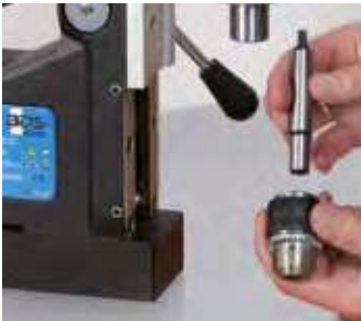
1. Connect taper drift to drill chuck.
