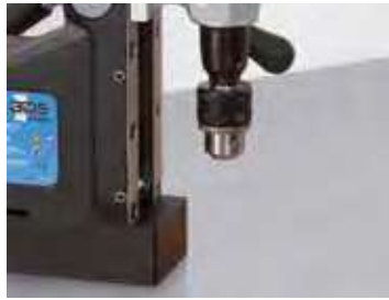
2. Insert drill chuck into the direct arbor.
