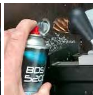
Step 2: During drilling, spray high-performance lubrication spray onto the tip of the drill and into the borehole.
